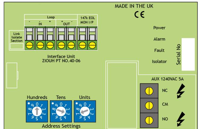
The unit has a built in loop short circuit isolator to help keep the unit operational in the event of a problem on the addressable loop wiring.
